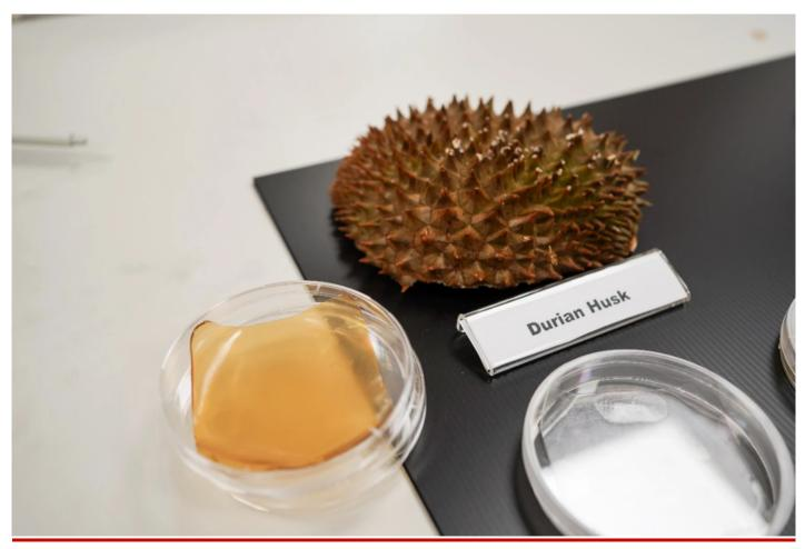
Durian husk and petri dish containing cellulose hydrogel sheet made out of durian husk with yeast phenolics are seen in Singapore September 16, 2021. Picture taken September 16, 2021.
